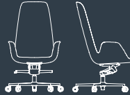
HALIA S0 YSYK MNGR 5SB/C/HA/5TM L: 745 mm / 29.3 inch D: 741 mm / 29.2 inch H: 1143-1228 mm / 45.0-48.3 inch
