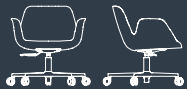
HALIA S0 YK OPR 5SB/C/HA/BM L: 745 mm / 29.3 inch D: 709 mm / 27.9 inch H: 978 - 1072 mm / 38.5 - 42.4 inch
